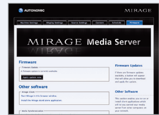
Figure 1: Remote Configuration Utility. For optimal performance and current features, install the latest firmware on your MMS-2 from the Firmware tab.
